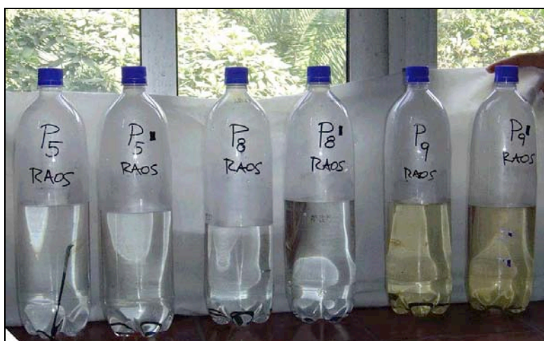
Figure 6 – PET bottles filled with arsenical solutions and cheap iron materials.
